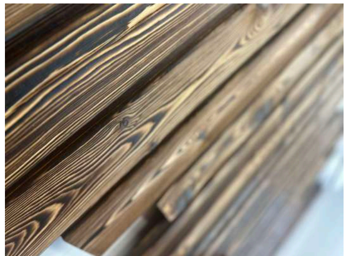
Image 2. Brushed charred wood cladding
